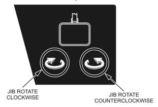
Figure 8-4. Jib Rotate Buttons (Detail)
